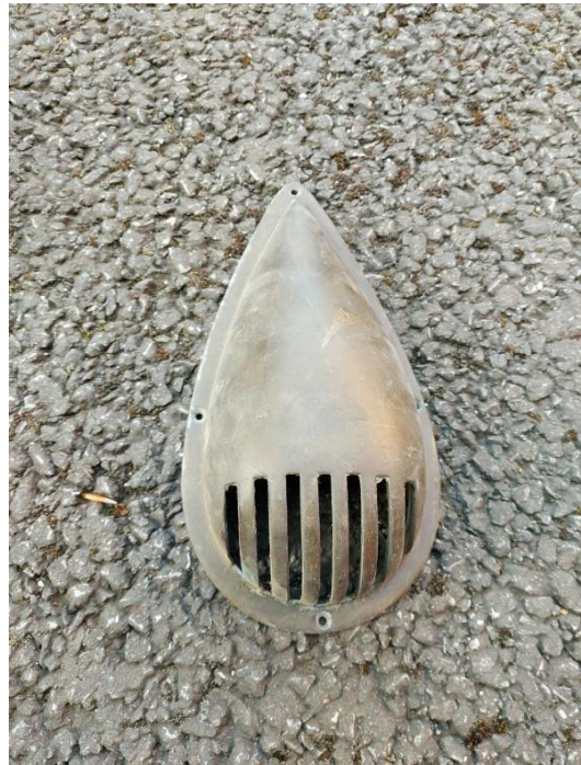
Item number #13. Navigation Light Cover Needs re-chrome and missing colour filter
