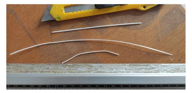
These strips are elastic enough to fit into window holes without breaking and adhere well to the shape of the wood. Here they are positioned after having slightly widened the openings, now the result is much better. I brought them to size and finished with sandpaper so that they are flush with the superstructure.
