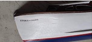
Here is a photo of the hull at present. I started applying very light strokes of glossy transparent water-based enamel on the mahogany and opaque parts on the bridge and sides.
