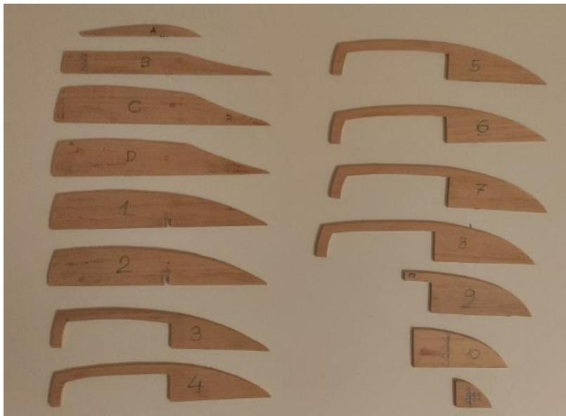
Later, I had to make some changes as Ben provided me with detailed drawings that are more accurate than I had so I realized that some part of the sections did not match. In particular, in sections 1 and 2 I had to move the floor step towards the bow and, from sections 3 to 9, I enlarged the cockpit-dinette space. In addition, Ben confirmed that there is a small step next to the helm seat and so I made this modification.
