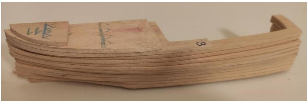
At this point, I proceeded to glue the sections starting from the hull and joining sections 1 and 2 separately from the others in order to refine the step more comfortably at a later time. As always, I used a vinyl glue (Vinavil).
