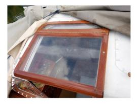
I prepare a sketch with the measurements then I glue some thin strips of mahogany Decoflex on an acetate rectangle, which I cover with paper tape so as not to scratch it during the subsequent activities (as has already happened with the windows.....)
