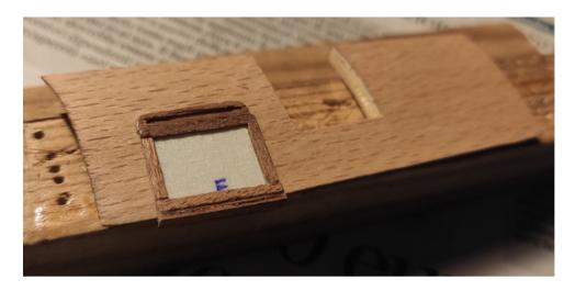
Then I round off the corners and smooth the wooden parts with sandpaper, then a light wash with white spirit and a little linseed oil to highlight the grain.
