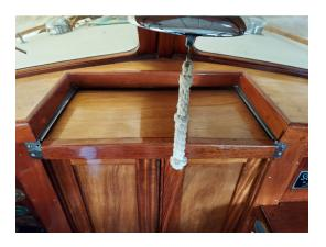
I must first put some support, which will later also be used for the windshield. So I use shaped and tailored wood scraps.
