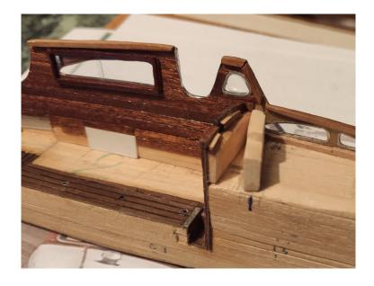
For the bottom I use a sheet of Decoflex beech wood while for the edges, slightly raised above the bottom, I use mahogany strips.
